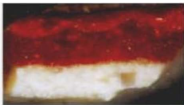
PLATE 26 The Ansidei Madonna (NG 1171). Cross-section from a mid-tone of Saint John's red drapery. The pale yellow imprimatura contains lead white, lead-tin yellow and powdered glass. Above are several red paint layers containing red lake, vermillion and powdered glass. Original magnification 480x; actual magnification 420x.
