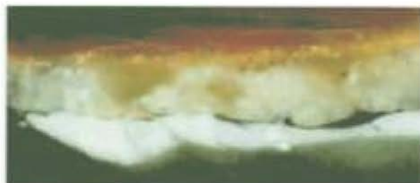
PLATE 21 The Procession to Calvary (NG 2919). Cross-section of Saint John's pale pink cloak. The thin uppermost red layers contain faded kermes red lake and vermilion. Beneath is a cream layer consisting of lead white, powdered glass and rounded translucent yellow particles that contain Al and Ca, and which are therefore very likely to be faded red lake (see PLATE 24). Below the cream layer is some black underdrawing, which lies on top of the pale yellow priming (lead white and lead-tin yellow). Original magnification 480x; actual magnification 420x.
