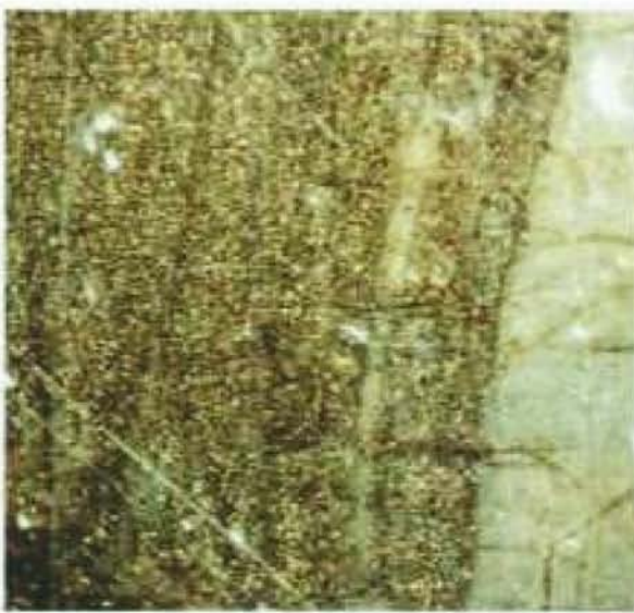
PLATE 39 The Madonna of the Pinks (NG 6596). Photomicrograph of the right edge of the dark grey tie of the chemise in PLATE 36, showing a pigment with a metallic lustre which has the characteristics of bismuth, 160x.
